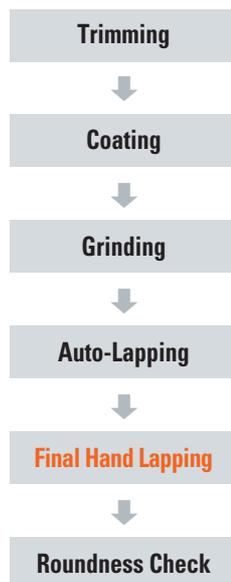
The surface of the parent material will be even after the trimming process, and blasting increases the adhesion of the coating.
